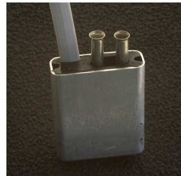
Textile LED module with and without fiber alignment ferrules
