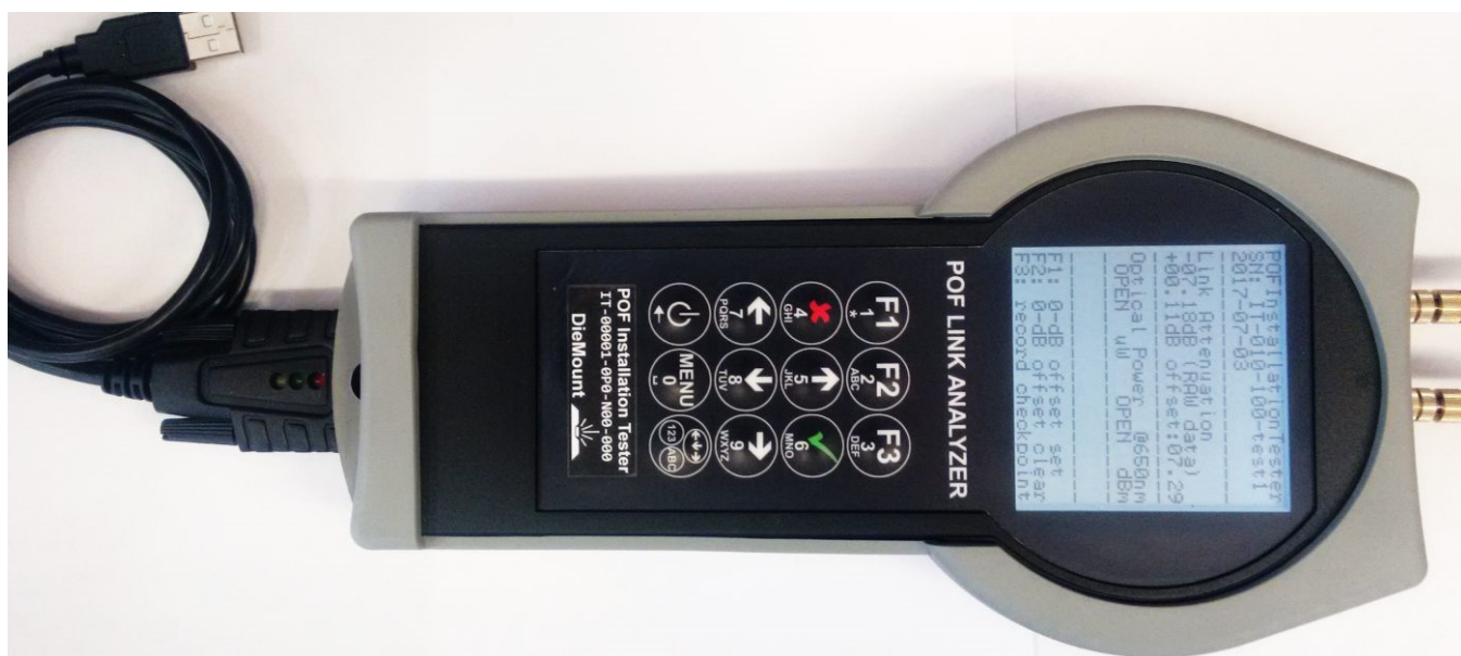
Figure 4. POF Link Analyzer in configuration as “POF Installation Tester” with USB cable and protective cover
