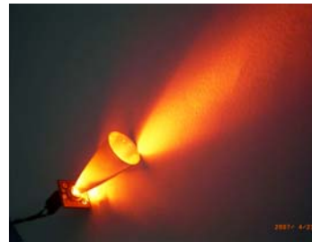
bare Spotlight LED in operation
