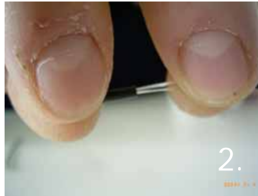
insertion to 2.2 mm POF cable
