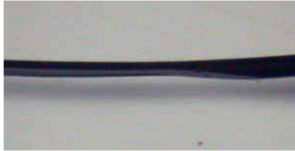
1mm POF (1.25 cable) polished to half diameter
