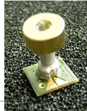
punched tube instead of extruded aluminium
